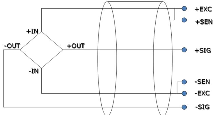
Note: short connect EXC1- and SEN1-, short connect EXC1+ and SEN1+ for 4 wires mode sensor.
