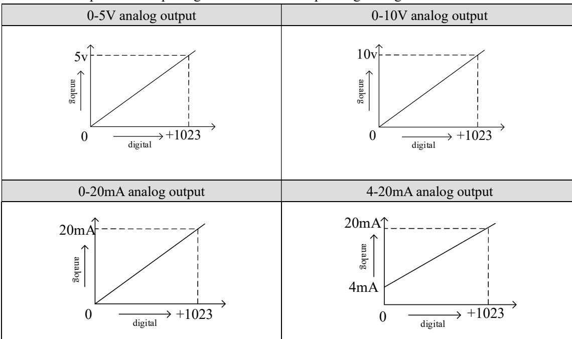
Note: When input data exceeds K1023, analog output will keep the value of 5V, 10V or 20mA.
