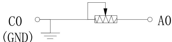
Note: the temperature input only supports two wire mode PT100 resistor input.
