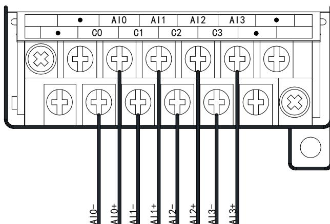
XD-E8AD-A current input wiring:
