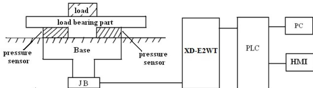
**Loading bearing part:** to support the load. Such as flat, hopper, container, air transport car...
