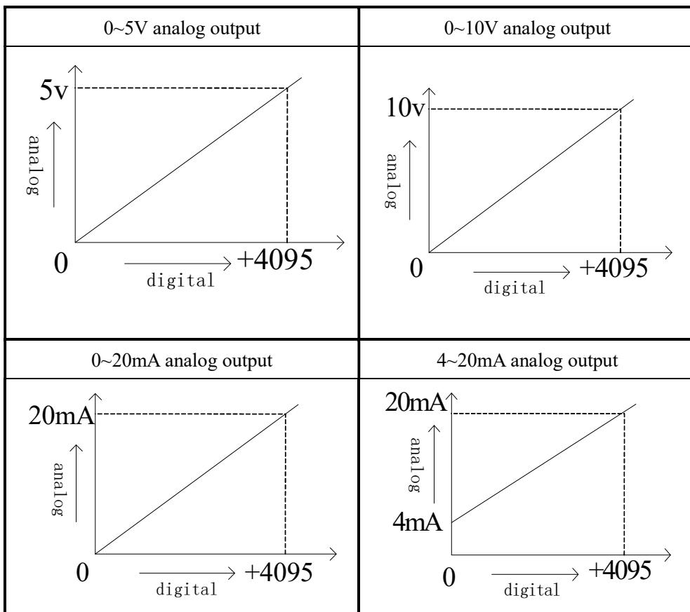
Note: when the input data exceeds K4095, the output analog data of D/A conversion remains unchanged at 5V, 10V or 20mA.
