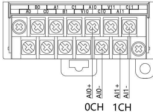
XD-E2AD2PT2DA current input wiring:
