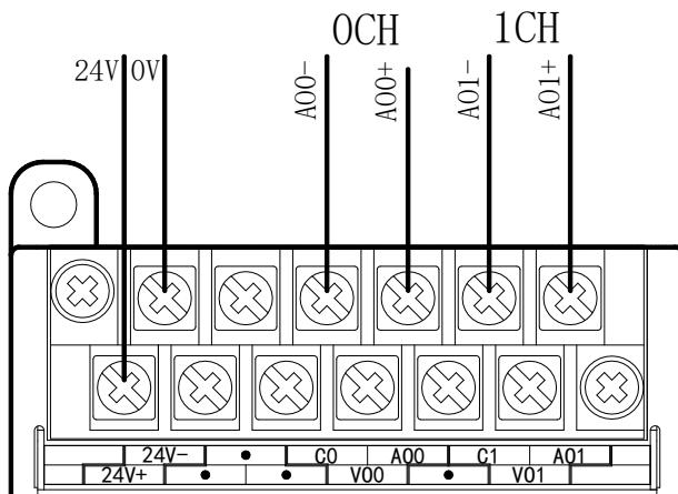
XD-E2DA current output wiring:
