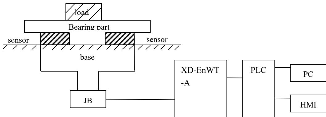
**Loading bearing part:** to support the load. Such as flat, hopper, container, air transport car...
