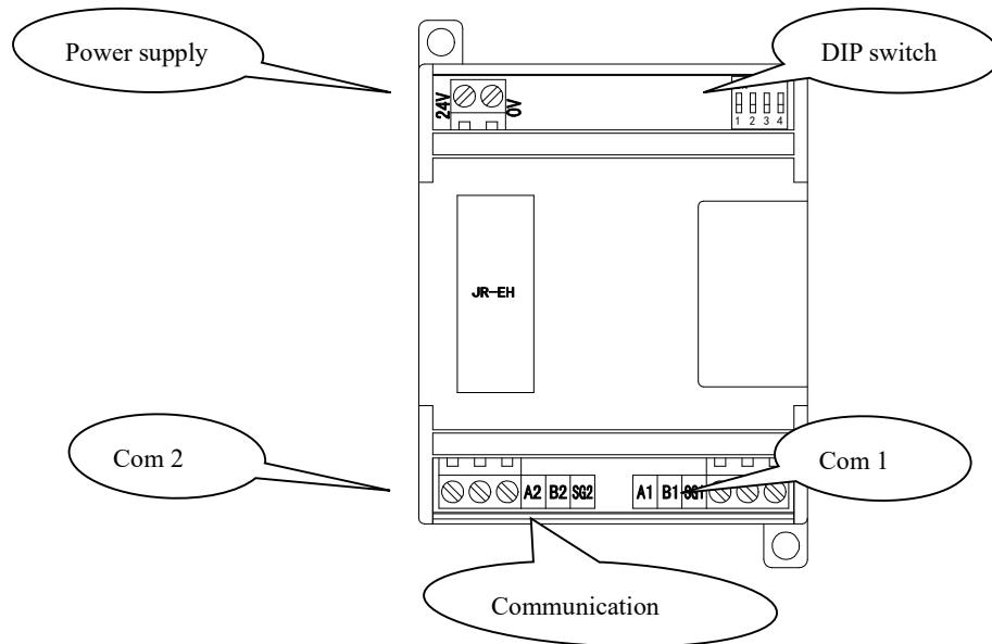
Com1 and com2 has no master and slave, they can be wiring as needs. Terminal A, B is for RS485, SG is ground terminal.
