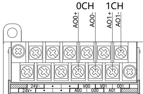
Note: the current output no needs to connect DC24V power supply.
