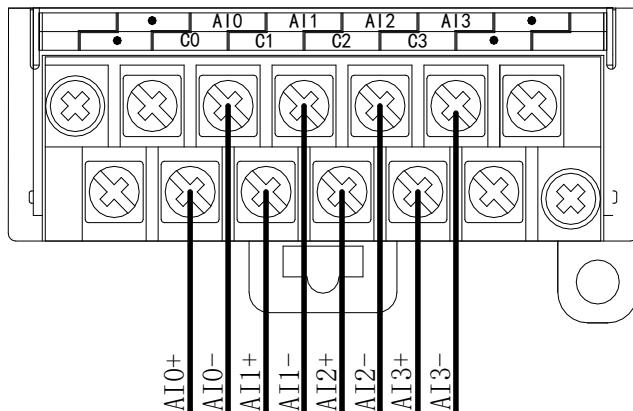
XD-E8AD current input wiring:
