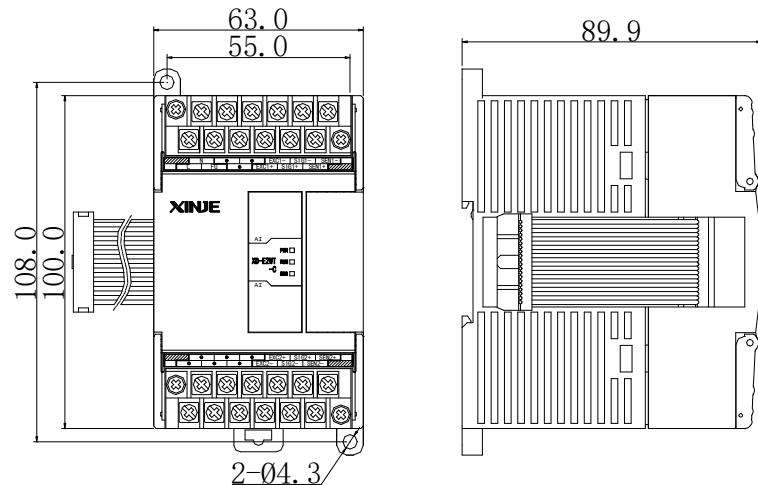
32 points I/O modules, XD-E4WT-C, XD-E4WT-D module: (dimension: mm)
