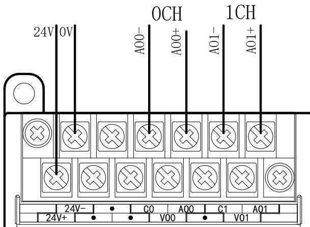
XD-E4DA current output wiring:
