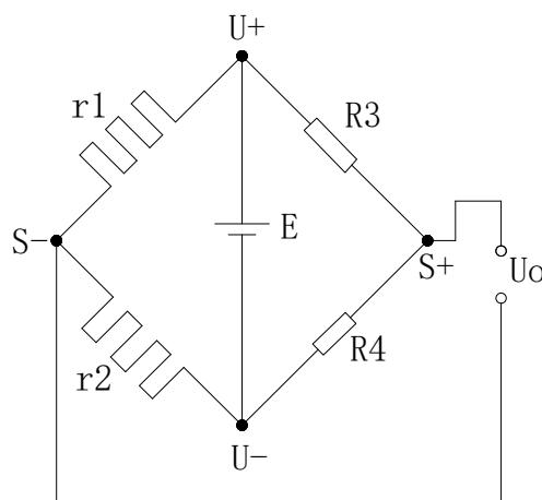
R1 and R2 is strain resistor which make bridge circuit with R3 and R4. With the change of R1 and R2, the bridge circuit will lose the balance, unbalance voltage  $U_o$  will be produced as the output of sensor.
