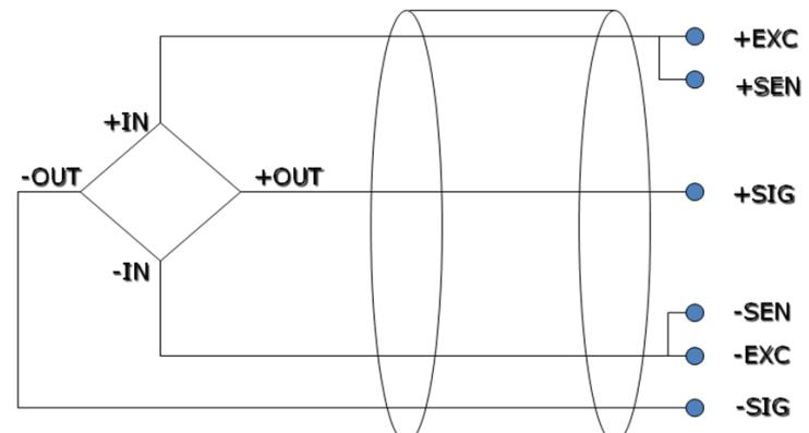
Note: short connect EXC1- and SEN1-, short connect EXC1+ and SEN1+ for 4 wires mode sensor.
