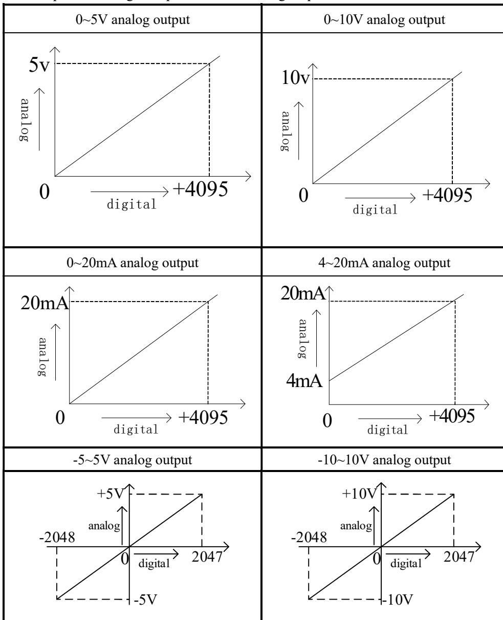
Note: when the input data exceeds K4095, the output analog data of D/A conversion remains unchanged at 5V, 10V or 20mA.
