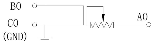
For the general three wire PT100 platinum thermistor, the wiring mode can be distinguished according to the wire color. The two wires of the same color can be randomly connected to terminal B0 and C0, and the other end can be connected to terminal A0.
