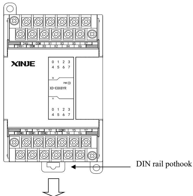
The module can be mounted on the DIN46277 rail (width 35mm). Pull down the DIN rail pothook to uninstall the module.
