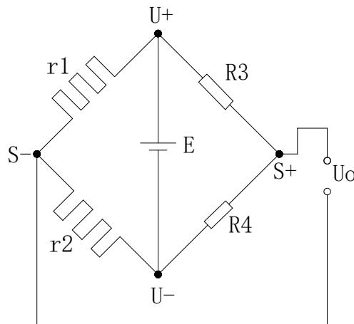
R1 and R2 is strain resistor which make bridge circuit with R3 and R4. With the change of R1 and R2, the
