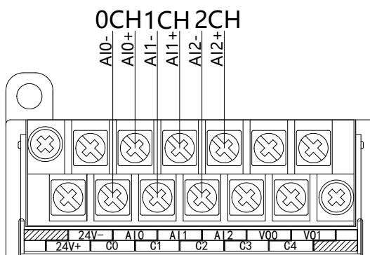
XD-E3AD4PT2DA current input wiring:
