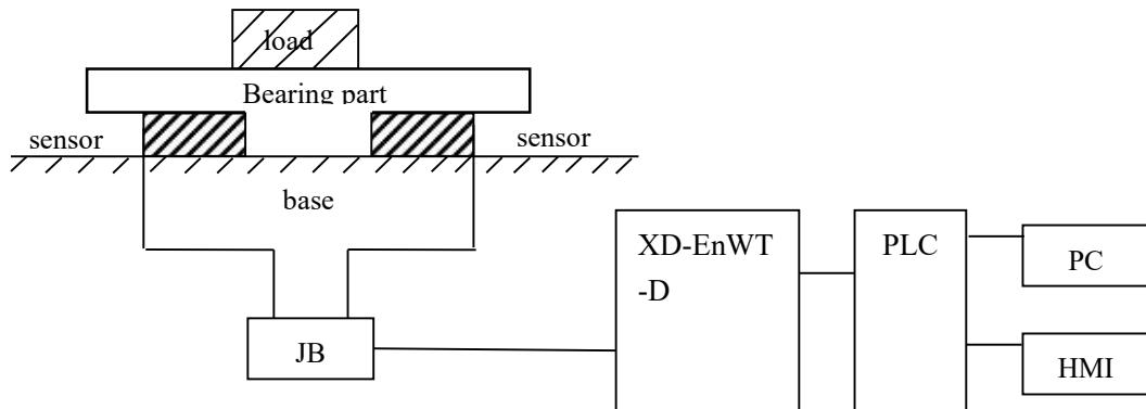
**Loading bearing part:** to support the load. Such as flat, hopper, container, air transport car...
