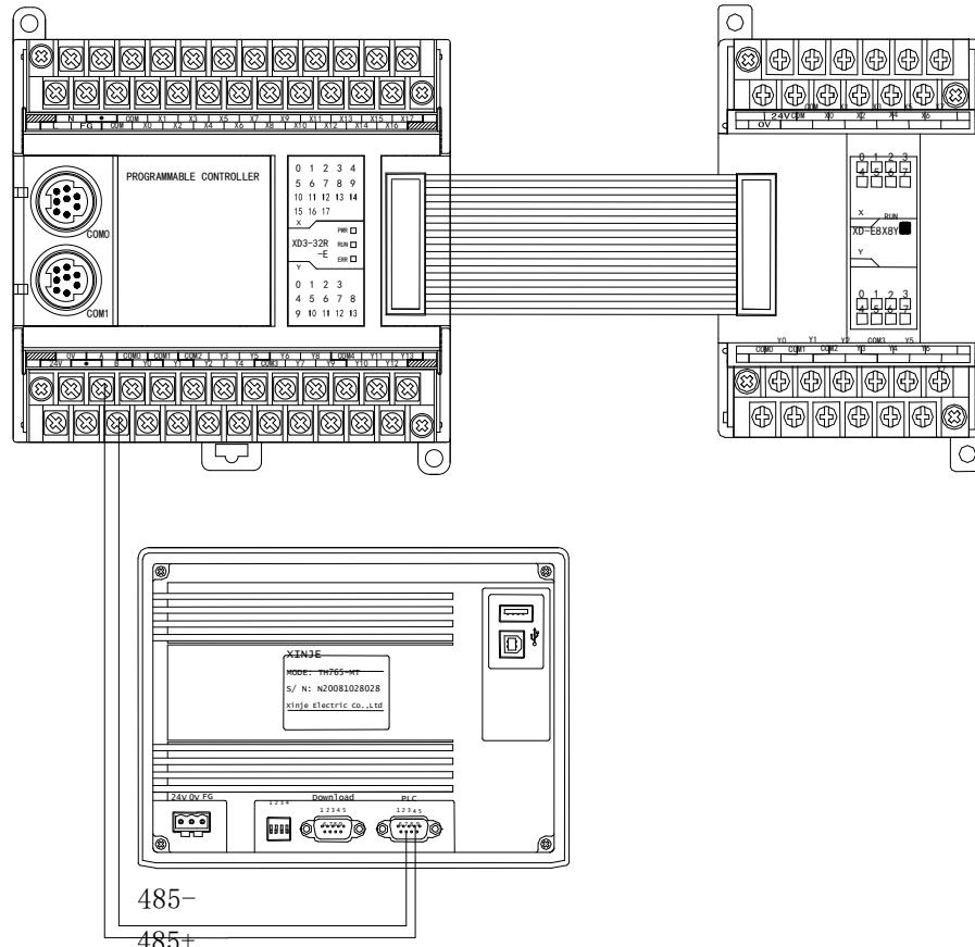
In this example, the HMI is the master station, read the input status of extension module to the HMI, writes the coil status of HMI to the extension module.
