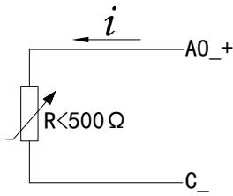
Note: There is no need to connect DC24 power supply in series for current output.
