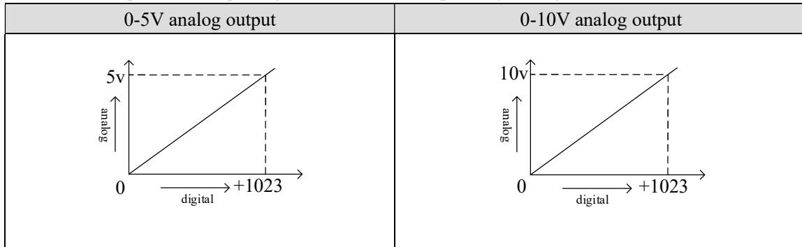
Note: When input data exceeds K1023, analog output will keep the value of 5V, 10V or 20mA.
