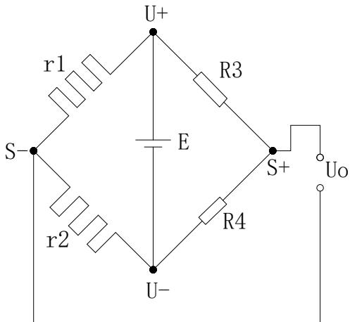
R1 and R2 are strain resistor which make bridge circuit with R3 and R4. With the change of R1 and R2, the bridge circuit will lose the balance, unbalance voltage  $U_o$  will be produced as the output of sensor.
