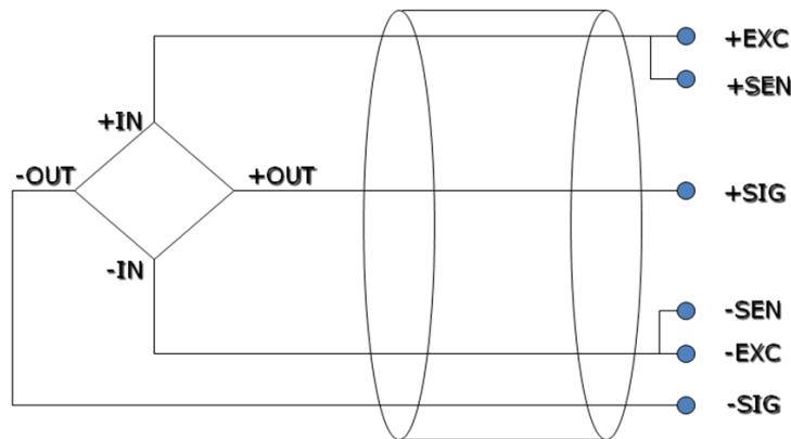
Note: short connect EXC- and SEN-, short connect EXC+ and SEN+ for 4 wires mode.
